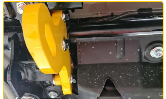
FIGURE 4: UNDERTRAY IN PLACE AFTER NOTCHING
