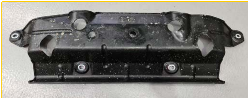
FIGURE 3: NOTCHING OF PLASTIC UNDERTRAY
