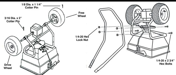
bve spreader and components from carton lace spreader upside down. Slide drive and wheels on axle as shown with the longer portion of wheel hub facing the frame. Secure free wheel with a 1/8 Dia. x 1 1/4" cotter pin. Secure drive wheel to axle with 3/16" Dia. x 2" cotter pin.
